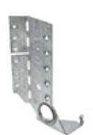
LSSJ™ Face-Mount Adjustable Jack Hanger Connecting jack rafters to hip members. Installs from one side with all fastener holes accessible. SKU# SIMLSSJ
