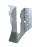
HTU Face-Mount Truss Hanger Full allowable loads (with minimum nailing) apply to heel heights as low as 3 7/8". SKU# SIMHTU
